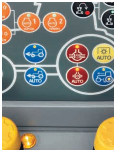
TerraLock controls for T7000 Sidewinder™ II models with electro-hydraulic rear remotes.
