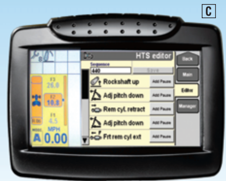
On Sidewinder™ II models, these switches (A) on the Intuitive Command Console are used to record a sequence of actions. Then, press the “CHM” button on the CommandGrip™ multi-function controller (B) to actually activate the recording or playback. Your programmed sequence appears on the IntelliView™ III screen (C). On Classic models, rocker switches allow you to record sequences and the transmission display keeps you informed.
