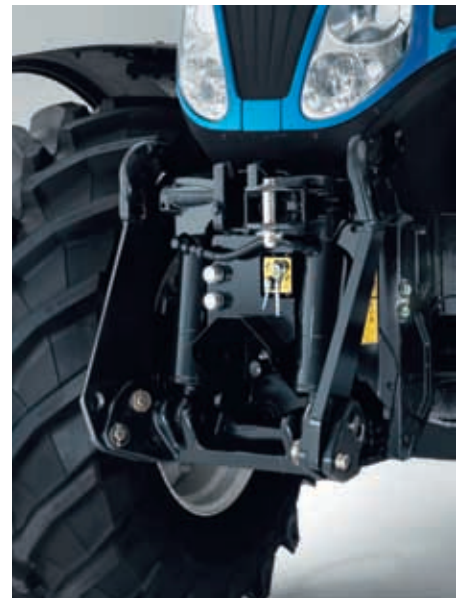
NEW front three-point hitch or front three-point hitch WITH PTO options allow you to power and control front-mounted implements for added versatility and the ability to double your productivity.
