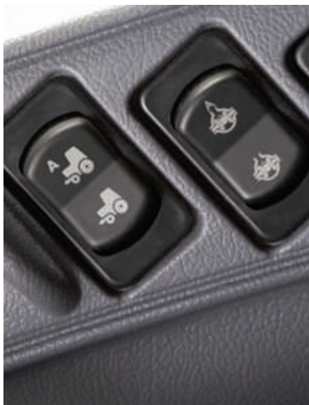
TerraLock™ controls for T7000 Classic models with mechanical rear remotes.
