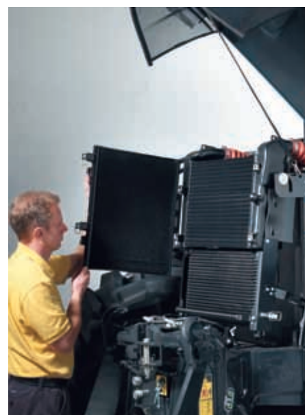
A flip-up hood with gas strut allows for fast and easy access to the radiator, A/C condenser and engine air filter.
