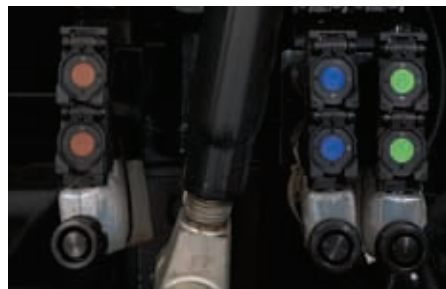
Hydraulic control levers and remote coupler dust covers are color-coded to assist with easy implement hook up and control.
