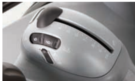
Electronic Draft Control is located for easy access and adjustment.
