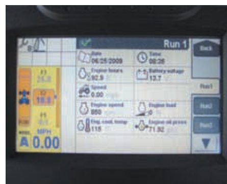
The IntelliView™ III display shows you the Auto Command™ target speed segment and operational mode you've selected.
