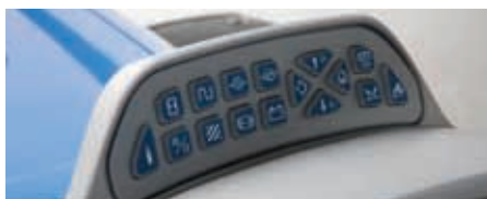
A standard enhanced keypad allows you to track engine hours and distance traveled, program service reminders and select the display modes that allow you to monitor tractor performance.
