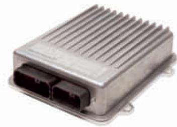
The Navigation Controller™ II receives user, satellite, correction and steering inputs and provides the control to guide the tractor. It includes three gyrometers.
