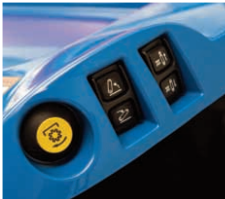
Switches for both the PTO and three-point hitch are provided on both rear fenders for easy control from the ground. Switches to control the #3 remote are also provided on models equipped with electro-hydraulic remotes.
