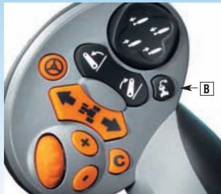
On Sidewinder™ II models, these switches (A) on the Intuitive Command Console are used to record a sequence of actions. Then, press the “CHM” button on the CommandGrip™ multi-function controller (B) to actually activate the recording or playback. Your programmed sequence appears on the IntelliView™ III screen (C). On Classic models, rocker switches allow you to record sequences and the transmission display keeps you informed.
