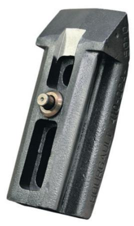
This heavy duty Speed-Loc<sup>™</sup> adapter fits all chisel plow 50° shanks except the Bourgault, the Morris Magnum III and the LH 755 shank on the Morris Concept 2000. The bottom bolt hole is slotted to fit 1-3/4 inch to 3 inch (45 mm to 77 mm) bolt spacing and it is mounted on the shank with 1/2 inch (12 mm) hex head bolts.
