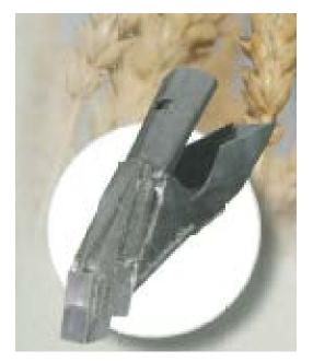
These 1" (25mm) vertical knives are our longest wearing openers. The high chrome cast tip has a double carbide insert that protects the bottom 2" (50mm) of the tip. Because of the near vertical approach, this opener will pull harder than conventional knives, however it will throw less soil and pull out fewer rocks.
