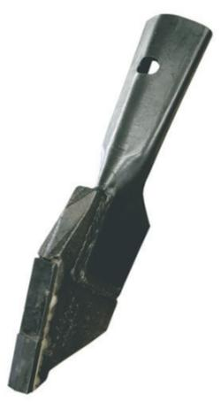
This knife has a 3/4 inch (19 mm) carbide tip welded to a 5/16 inch (8 mm) quick change holder. In addition to the bottom carbide insert there is also a secondary carbide insert to prevent the cast tip from wearing above the primary carbide. The tip has a 75° approach angle which means that it will not lift and pull many rocks or stumps to the surface.
