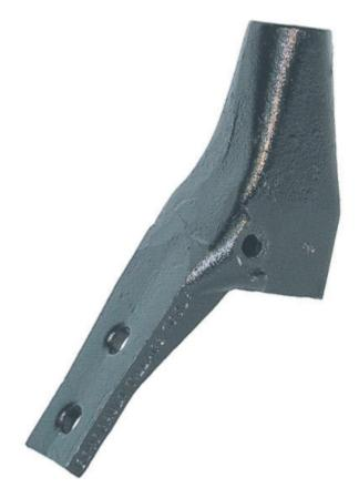
This holder has 1-3/4 inch (45 mm) bolt hole spacing. The bolt hole section is designed flat to fit the Bourgault and Ezee-On 47° shanks.
